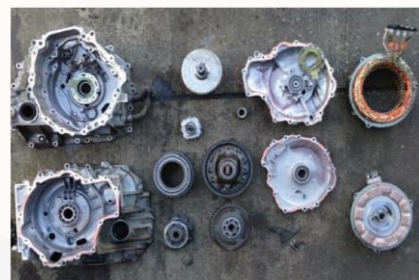
REE magnets rotor Manual pre-dismantling
