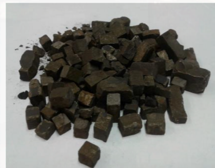
NdFeB magnets Feed of the hydro process
