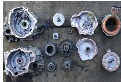
REE magnets rotor Manual pre-dismantling
