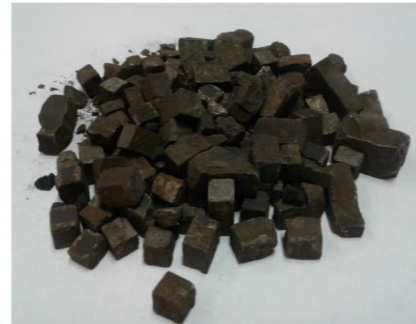
NdFeB magnets Feed of the hydro process
