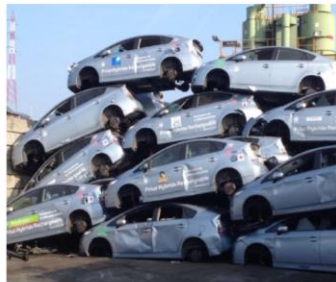
Depolluted hybrid vehicles 1.2 kg of magnets/vehicle
